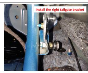
9. Install the right tailgate bracket on the right hinge.
