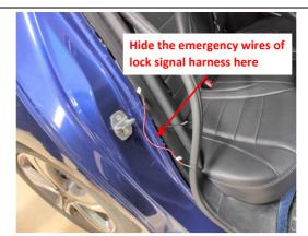
19. Route the emergency wires of the lock signal harness to the right side of rear seat (the emergency wires should be in 20. Ground at the right side of the trunk with the ground place for emergency use).
