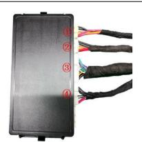
27. Insert the strut wiring harnesses (1)(2), lock signal harness (3), and power harness (4) into the ECU in sequence.
