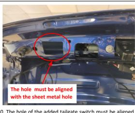
30. The hole of the added tailgate switch must be aligned with the sheet metal hole.
