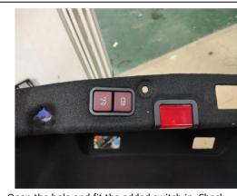
31. Open the hole and fit the added switch in. Check whether the buttons can bounce back normally when pressed and then reinstall all the trim panels
