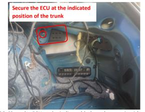
26. Place the ECU at the indicated hole and secure it with a
