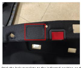
29. Stick the hole template to the indicated position on the tailgate trim panel.
