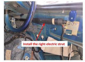
11. Install the right electric strut, L on the left and R on the right (the first letter of the strut code), making sure the end with wiring harness pointing outward.
