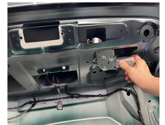
16. Put the power latch into the tailgate from the right side of the tailgate.
