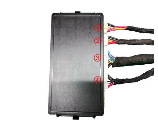
27. Insert the left and right strut wiring harnesses ①②, lock signal harness ③, and power harness ④ into the ECU in sequence.
