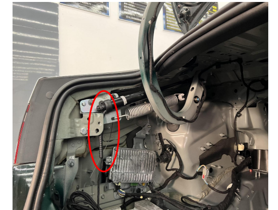
11. Install the electric struts with L on the left and R on the right (the first letter of the strut code).
