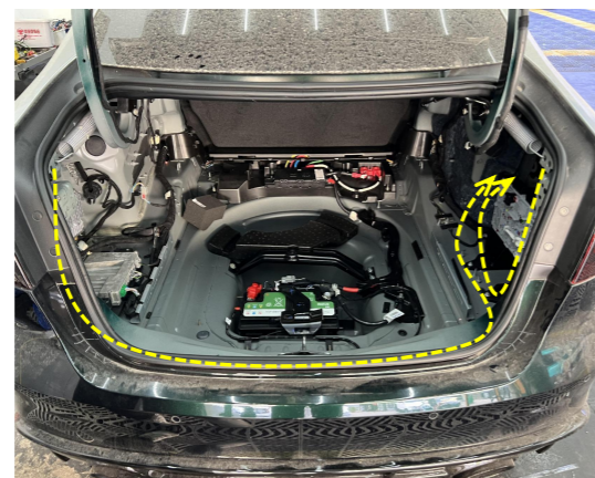
13. Route the strut wiring harnesses to the right side of the trunk along the original wiring harnesses.
