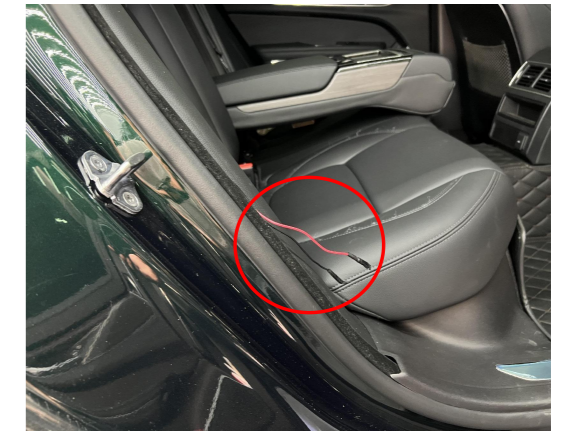
21. Route the two emergency wires of lock signal harness to the right side of the rear seat and hide them under the trim.
