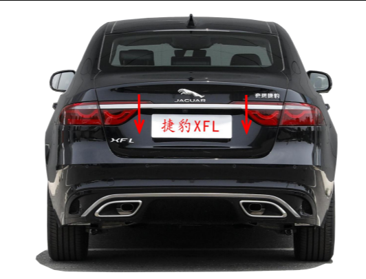
29. Press the original tailgate switch button to open the tailgate for initialization and test each function of the electric tailgate.
