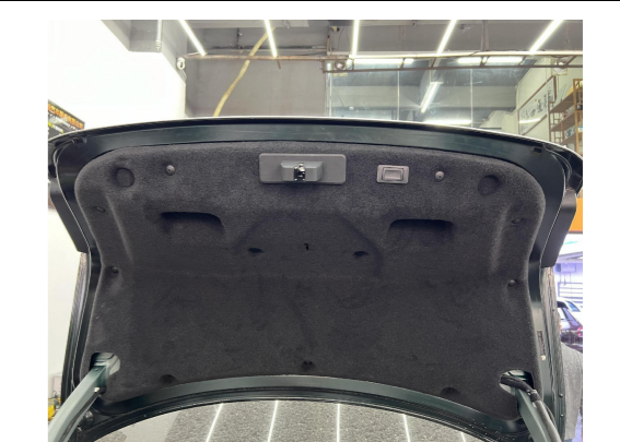
31. Install the added tailgate switch, cover the latch with provided plastic casing and reinstall all trim panels.
