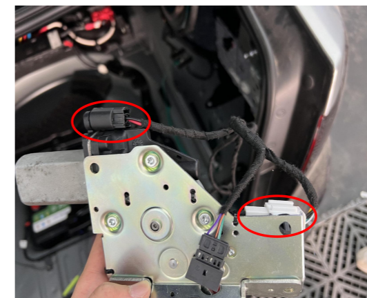
15. Connect the lock signal harness to the plugs of our power latch.
