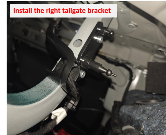
10. Install the right tailgate bracket with the ball stud on the upper side and add two washers.
