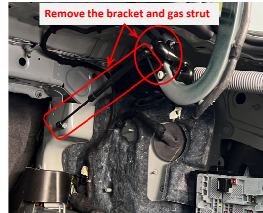
9. Remove the bracket used for hanging spring from the right hinge and remove the gas strut.
