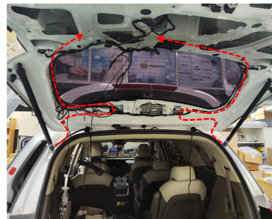
9. Thread the wiring harnesses through the holes into the tailgate and route them as indicated.
