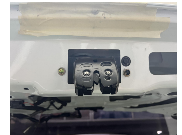
11. Remove the original latch and install our power latch.
