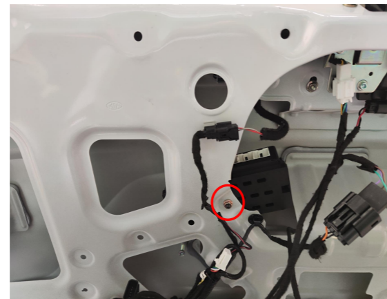
22. Secure the ECU at the indicated position of the tailgate.
