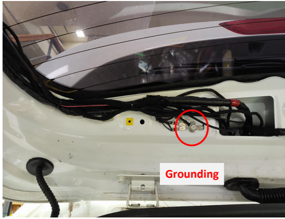
17. Ground at the indicated position on the tailgate.
