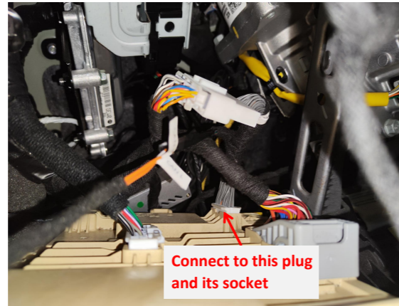
18. Connect to the indicated CAN plug and its socket behind the fuse box.
