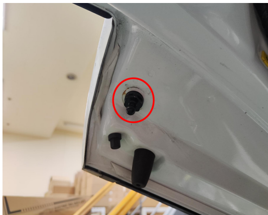
7. Replace the tailgate ball studs.
