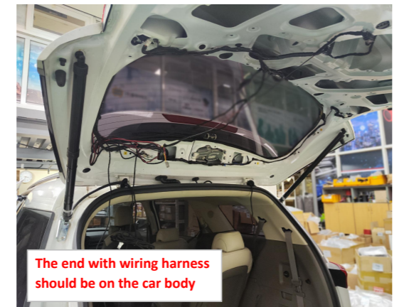
8. Install the electric struts, L on the left and R on the right (the first letter of the strut code).
