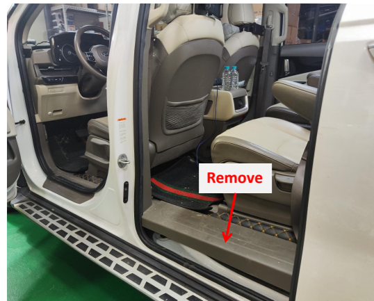
2. Remove the middle door step board.
