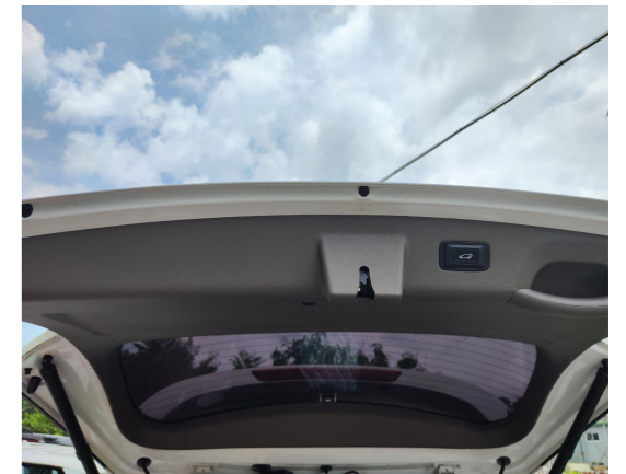
25. Install the added tailgate switch and reinstall all the trim panels.
