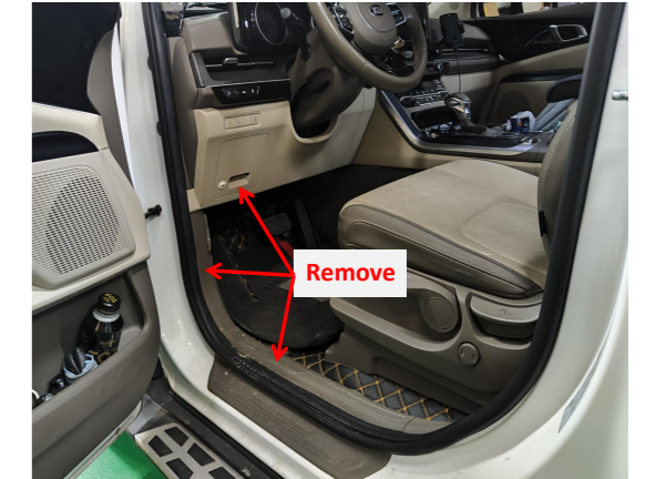
1. Remove the fuse box trim panel and door sill panels as indicated.
