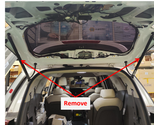
4. Remove the original gas struts.
