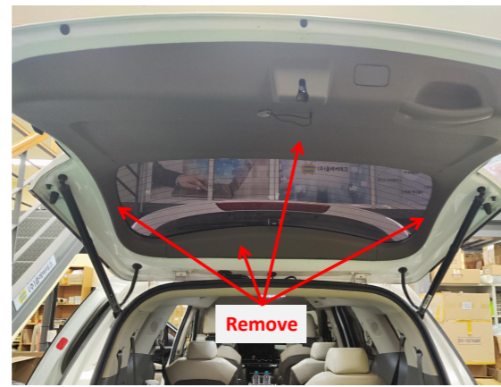
3. Remove the tailgate trim panels.
