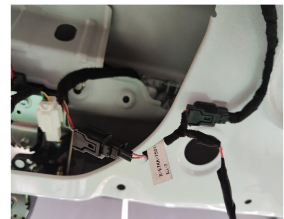
13. Connect the plugs of the lock signal harness to the plugs of original tailgate switch.
