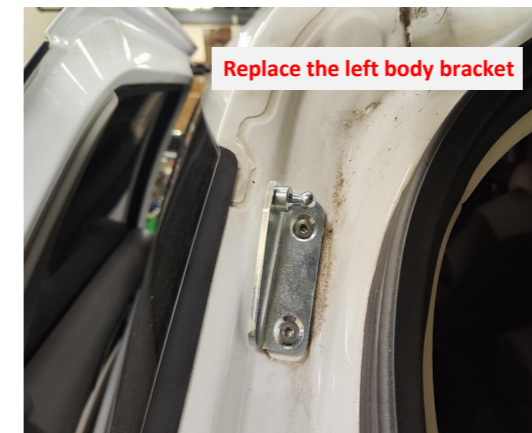
5. Replace the left body bracket.
