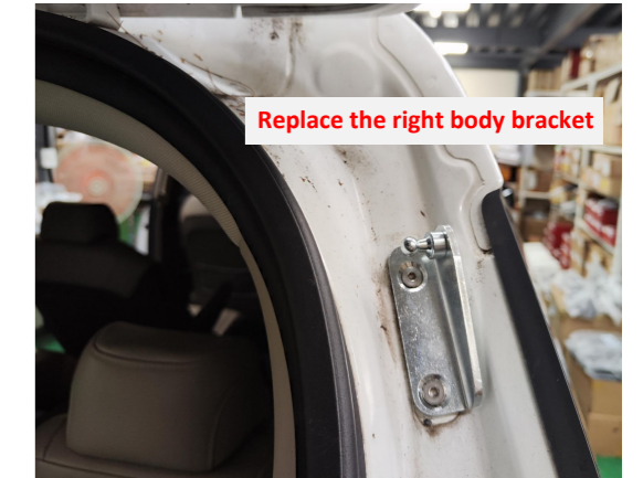
6. Replace the right body bracket.
