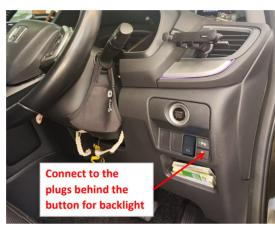
23. Connect the power harness to the plugs of the front switch behind the panel.
