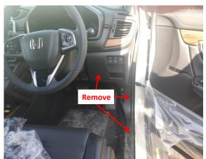
1. Remove the indicated front right side trim panels and door sill panel.
