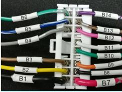
Note: For models with fewer than 14 wires, just insert them according to the corresponding label or color. 15. Insert the lock signal harness termianls into the wiring
