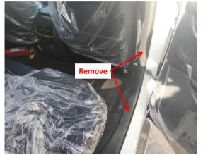
. Remove the rear right side door sill panel and B-pillar trim 3. Take out the trunk floor mat and remove the trim panel panel on the right side of the trunk.
