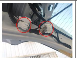
17. Connect the plug of the lock signal harness to the plug of 18. Connect the plugs of the lock signal harness to the plugs the added tailgate switch. of the tailgate handle switch.
