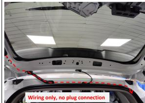
14. Thread the lock signal harness to the right side of the trunk.
