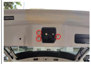
13. Remove the original latch and install the power latch.
