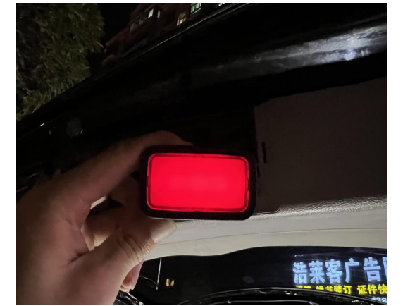
21. Connect the handle light to its plug and put it inside the tailgate trim panel.
