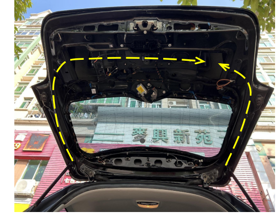
6. Thread the left and right strut wire harnesses through the drilled holes into the tailgate.
