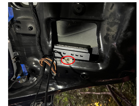
16. Install the ECU and secure it with a nut (the nut is located on ECU).
