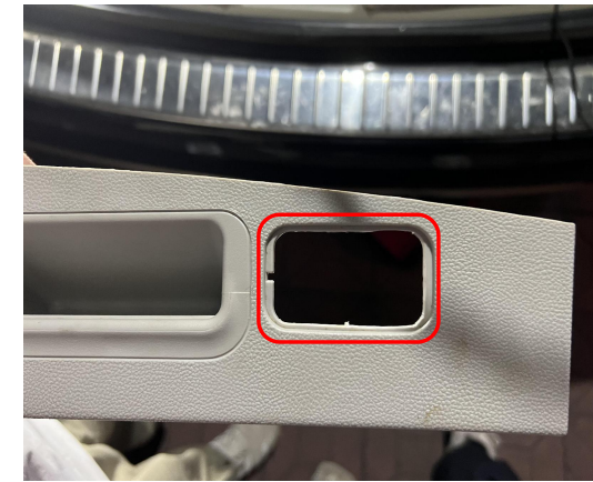
20. Remove the tailgate handle light and adjust the hole size to fit the added switch.
