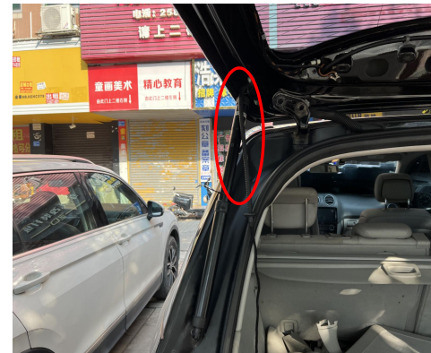
4. Install the electric struts, L on the left and R on the right (the first letter of the strut code), making sure the ends with wire harnesses are on the tailgate.
