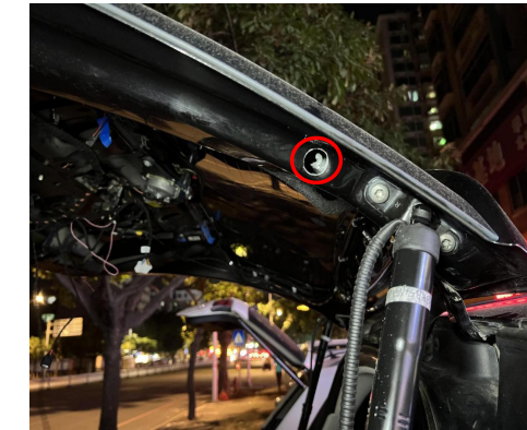
5. Drill a hole at the indicated location with a \phi 21 mm drill bit to allow the strut wire harness to pass through. Both sides are the same.
