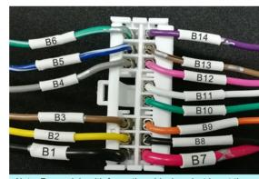
Note: For models with fewer than 14 wires, just insert them according to the corresponding label or color. 9. Insert the lock signal harness terminals into the wiring
