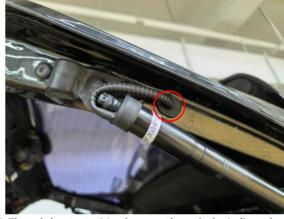
5. Thread the strut wiring harness through the indicated hole into tailgate and plug the hole with hole plug.
