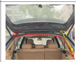
6. Route the strut wiring harnesses to the right side of the
