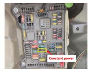
13. The fuse slot for power supply is indicated above.
