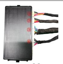
17. Insert the strut wiring harnesses (1)(2), lock signal harness (3), and power harness (4) into the ECU in sequence.
