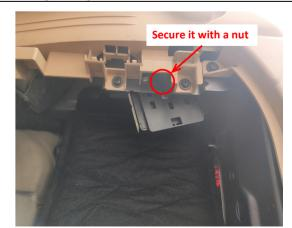
16. Secure the ECU to the indicated hole at the right side of the trunk with a nut.
