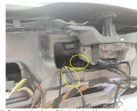
11. Connect the plugs of the lock signal harness to the plugs of the original tailgate switch and the added switch.
