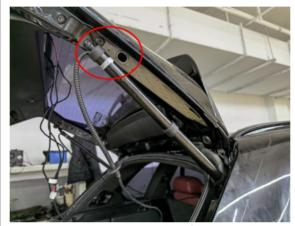
I. Install the electric struts, L on the left and R on the right (the first letter of the strut code).
