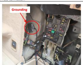
12. Ground at the right side of the trunk with the ground wire connector.
