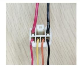
7. Insert the strut wiring harness terminals into the wiring harness connector.
