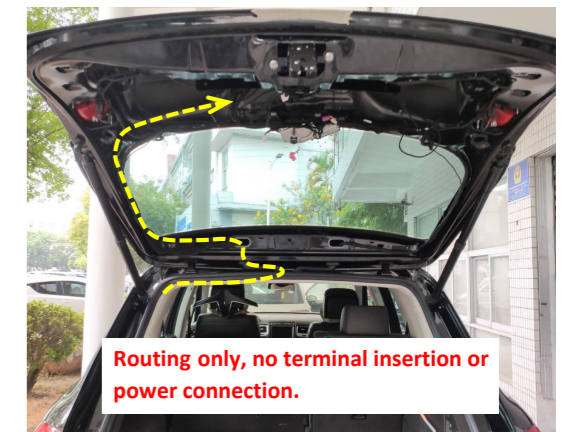
16. Route the power harness as indicated (routing only, no terminal insertion or power connection.)
