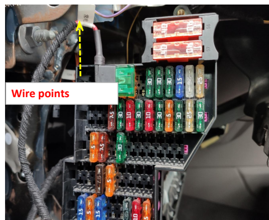
22. Plug the fuse tap into the fuse box and pay attention to the direction of wire.
