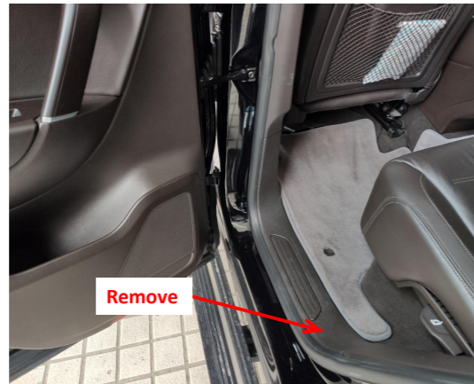
3. Remove the rear left door sill panel.
