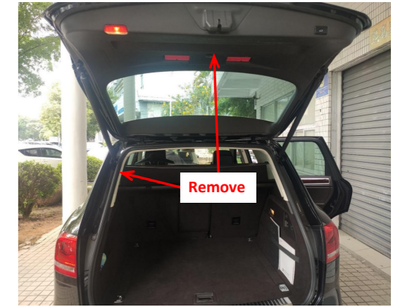
1. Remove the tailgate and trunk trim panels.
