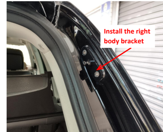
5. Install the right body bracket.
