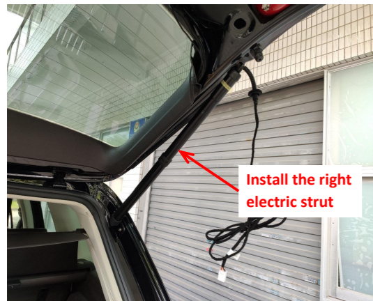
7. Install the right electric strut, L on the left and R on the right (the first letter of the strut code).
