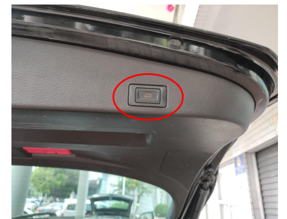
26. Install the added tailgate switch and reinstall all the trim panels. (remove the original small cover)
