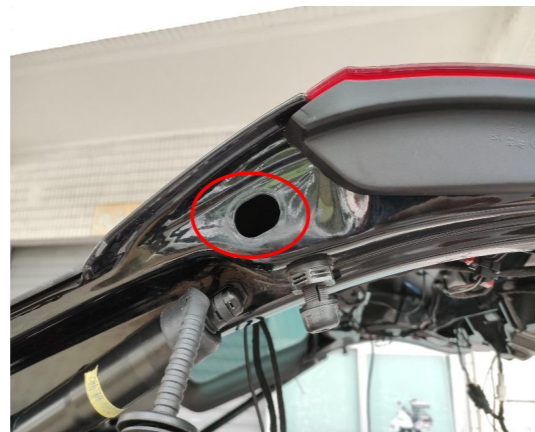
8. Thread the strut wiring harnesses into the tailgate through the indicated holes on both sides.
