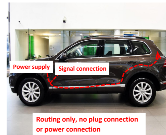
15. Route the power harness as indicated.
