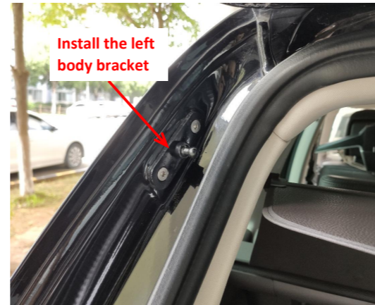
4. Remove the original gas struts and install the left body bracket.
