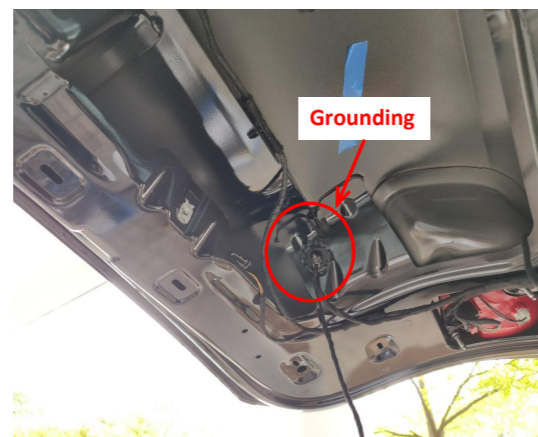
18. Ground at the indicated position of the tailgate.
