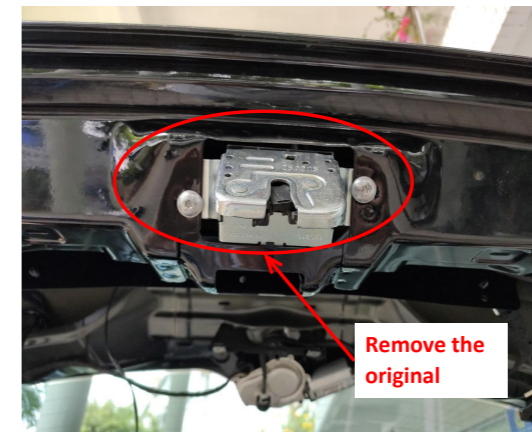
10. Remove the original latch.
