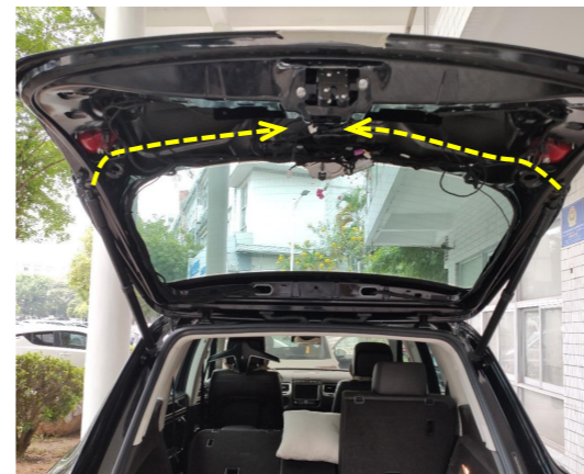
9. Route the left and right strut wiring harness as indicated and plug those two holes with hole plugs.
