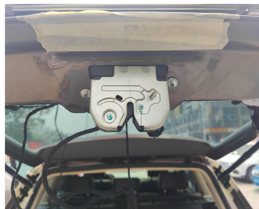
13. Install the power latch.
