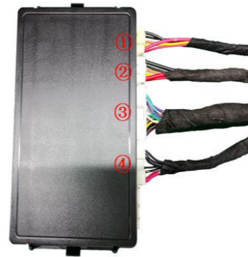
24. Insert the left and right strut wiring harnesses ①②, lock signal harness ③, and power harness ④ into the ECU in sequence.
