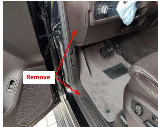
2. Remove the driver's side door sill panel and the indicated trim panel.
