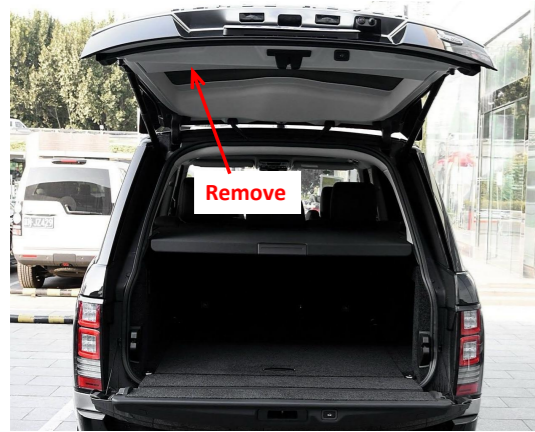
2. Remove the tailgate trim panels.
