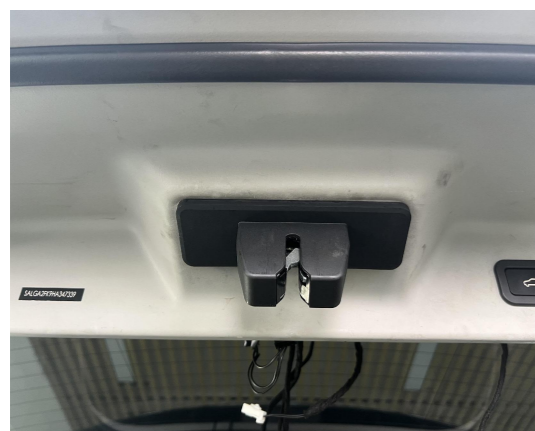
12. Install the power latch with the provided latch cover.
