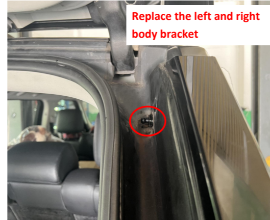
4. Replace the ball studs on both sides of the trunk.
