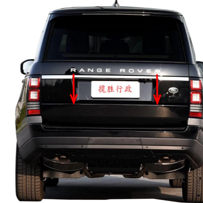
25. Press the added tailgate switch to close the tailgate once, the system completes initialization, and then test each function of the electric tailgate.
