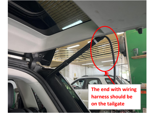
6. Install the electric struts, L on the left and R on the right (the first letter of the strut code).
