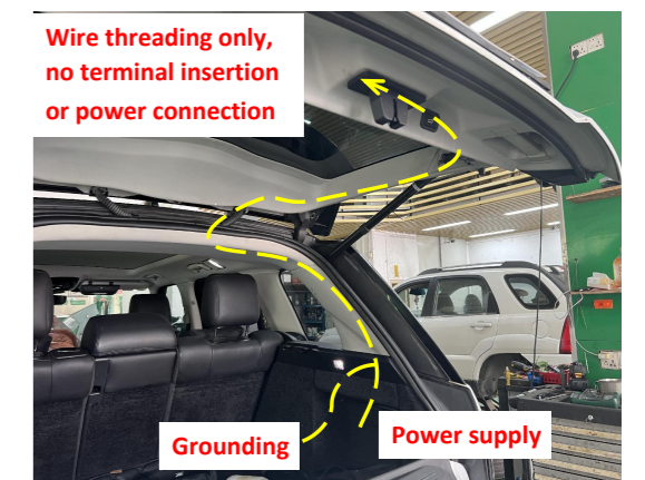
16. Route the power harness to the tailgate.
