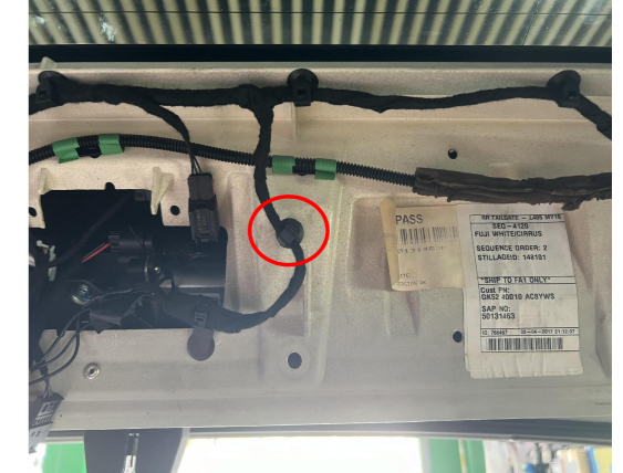
21. Remove the indicated cable clip.
