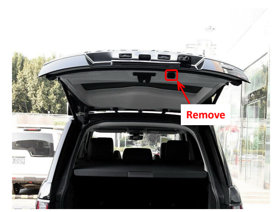
26. Remove the indicated small panel.
