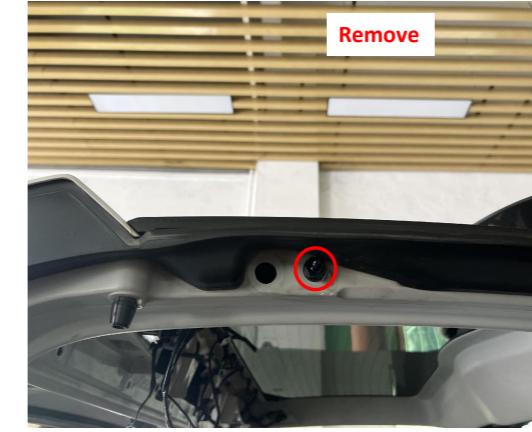
5. Replace the ball studs on both sides of the tailgate.
