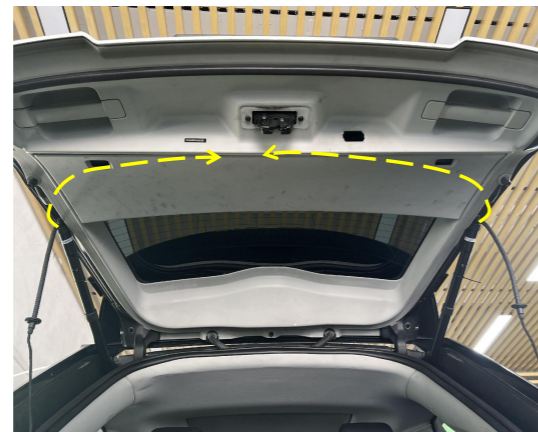
8. Route the left and right strut wiring harness as indicated.
