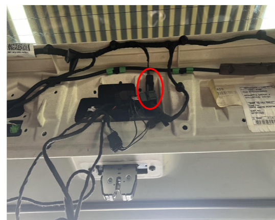
13. Connect the plugs of the lock signal harness to the plugs of original tailgate switch.
