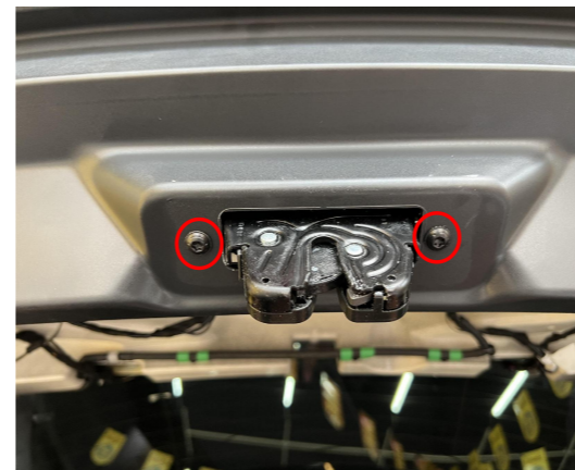
9. Remove the original latch.
