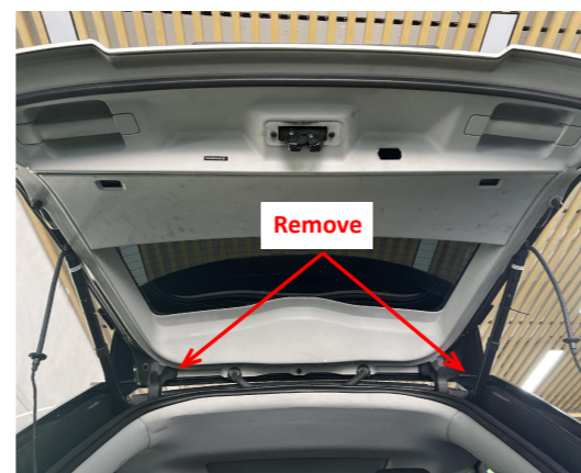
14. Remove the trim panels of the hinges.
