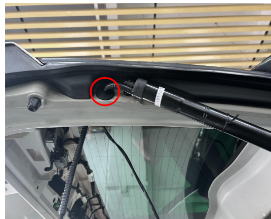
7. Thread the strut wiring harness through the indicated hole into the tailgate.
