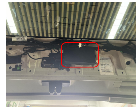
23. Mount the ECU onto it bracket.
