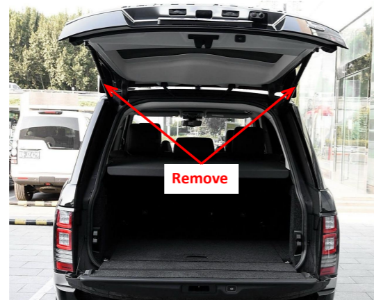
3. Remove the original gas struts.
