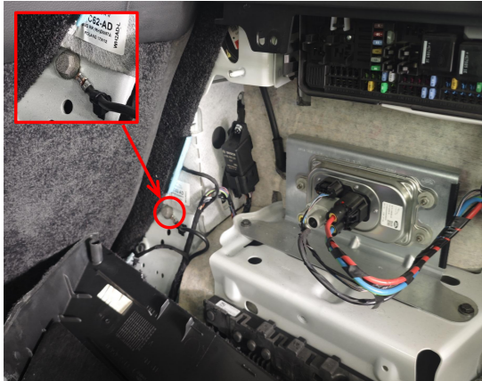
17. Ground at the indicated position on the right side of the trunk.
