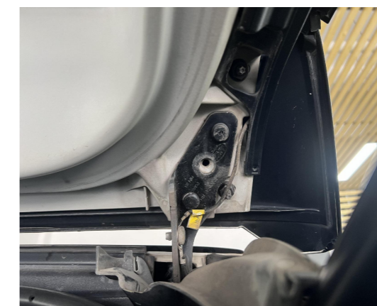
15. Remove the screw from the spoiler.
