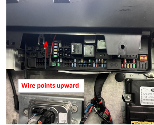
20. Plug the fuse tap into the fuse box and pay attention to the direction.
