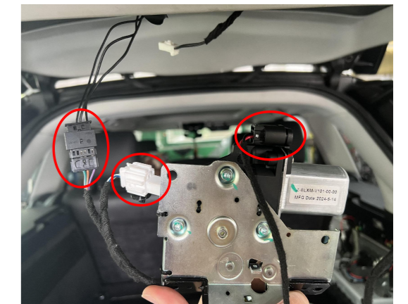
11. Connect the plugs of the lock signal harness to the plugs of the power latch.
