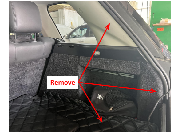
1. Remove the trim panels from the right side of the trunk.
