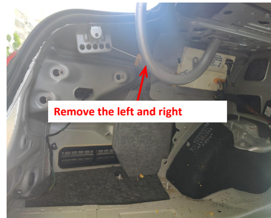
2. Remove the springs on both sides of the trunk.
