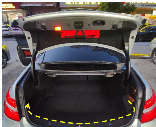
22. Route the power harness to the left side of the trunk.
