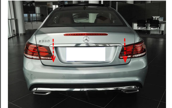
26. Manually close the tailgate to the position where it just touches the striker, then open the tailgate with the original tailgate switch to complete system initialization, and test each function of the electric tailgate.
