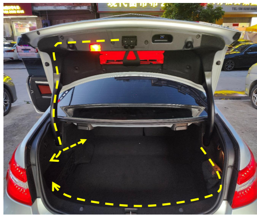
17. Route the lock signal harness and the right strut wiring harness to the ECU's location.
