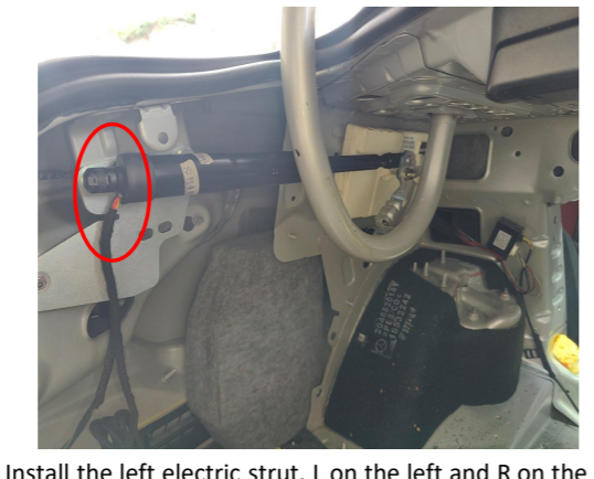
8. Install the left electric strut, L on the left and R on the right (the first letter of the strut code), making sure the end with wiring harness points outward.
