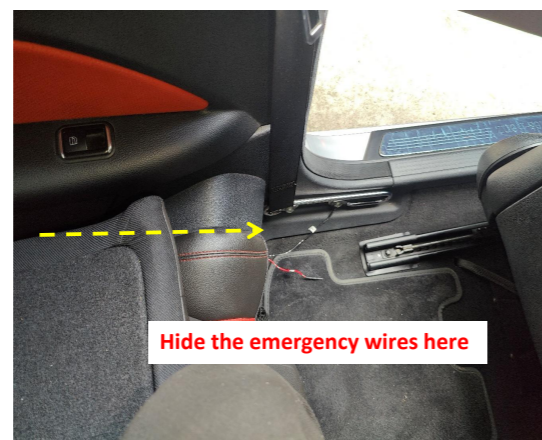
18. Route the emergency wires from the trunk to the left side of the rear seat and hide them here.
