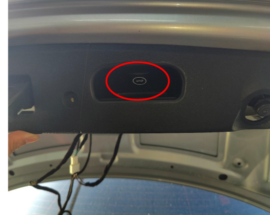
28. Install the added tailgate switch and reinstall all the trim panels.
