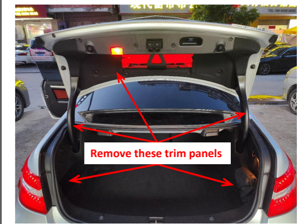
1. Remove the indicated trim panels from the tailgate, hinges and trunk.
