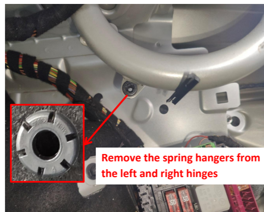
3. Remove the spring hangers from the left and right hinges.
