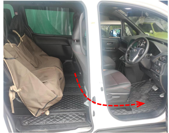
25. Route the front switch wiring harness and the signal plugs to the driver's area.
