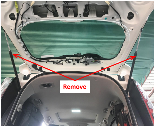
6. Remove the original gas struts.
