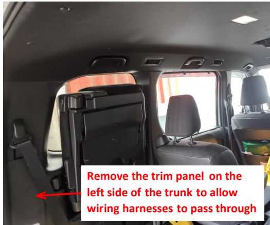
5. Remove the trim panel on the left side of the trunk to allow wiring harnesses to pass through.
