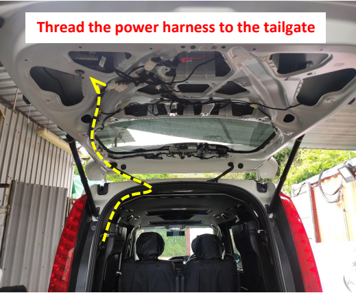
22. Thread the power harness to the tailgate.
