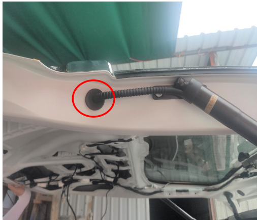
17. Plug the holes on the left and right sides of the tailgate with the hole plugs.
