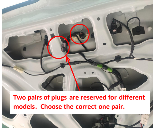
19. Connect the plugs of the lock signal harness to the plugs of the original tailgate switch.
