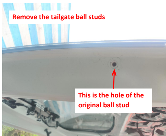
9. Remove the left and right ball studs.
