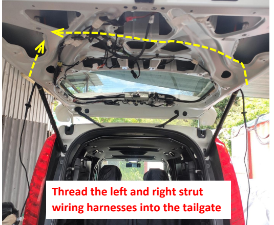
16. Thread the left and right strut wiring harnesses into the tailgate.
