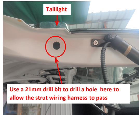
15. Use a 21mm drill bit to drill a hole here to allow the strut wiring harness to pass through. Both sides are the same.
