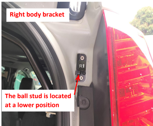
8. Mount the bracket at the right side of the trunk and pay attention to the position of the ball stud.
