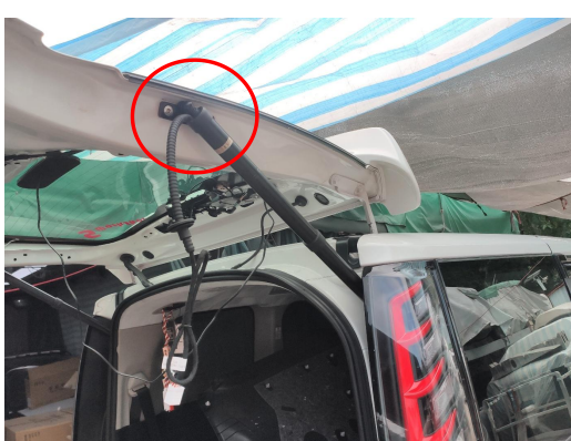
14. Install the electric struts, L on the left and R on the right (the first letter of the strut code), making sure the ends with wiring harness are on the tailgate.
