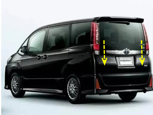
32. Press the added tailgate switch to open and close the tailgate once for initializing the system, and then test each function of the electric tailgate.
