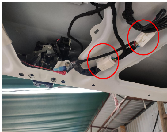
18. Connect the plugs of the lock signal harness to the plugs of the power latch.
