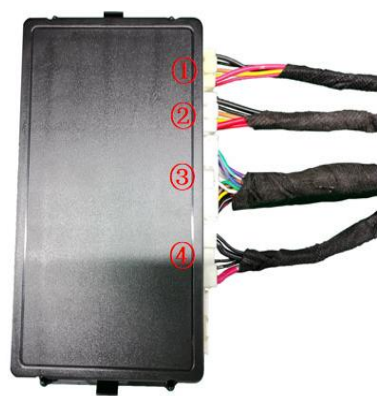
31. Insert the strut wiring harnesses ①②, lock signal harness ③, and power harness ④ into the ECU in sequence, and mount the ECU on its bracket.
