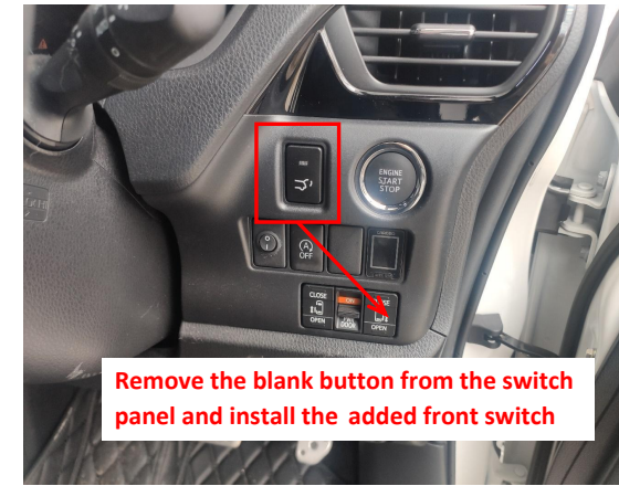
26. Remove the blank button from the switch panel and install the added front switch.
