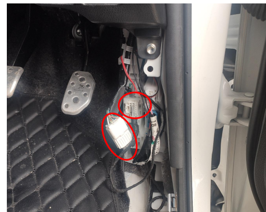
28. Connect the signal plugs of the power harness to the indicated plug and its socket beside the pedals.
