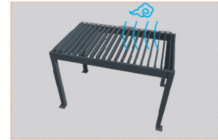
0-120°的叶片开合角度 通过折射实现调光 The blade opening and closing angle of 0-120° realizes the dimming function.
