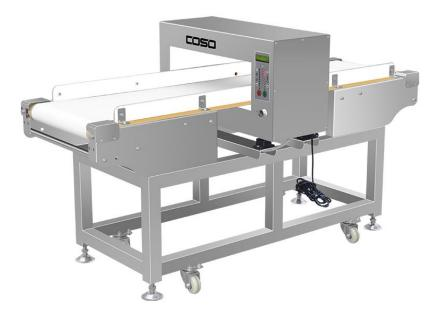
AMC500 metal detector specializes for non-Fe metallic film packing products, like foil aluminum, aluminum film, using magnetic induction principle to detect metallic impurities in aluminum foil packing food products. But this model machine can only detect out ferrous metal. Machine can't detect non-fe and Stainless steel from products.
