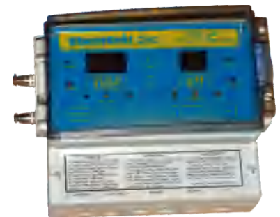
Water quality monitor monitors PH/(residual chlorine)
