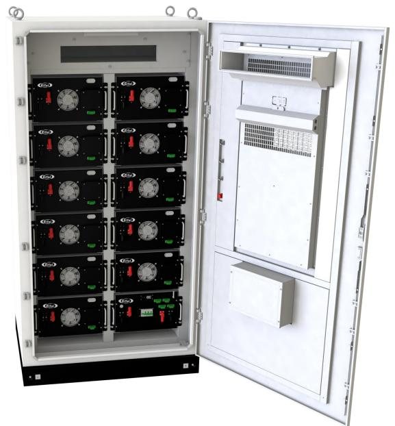
EITAI-HV high voltage lithium battery energy storage system, consisting of 6-11 battery modules (51.2V200Ah) and a BCU (Battery Control Unit) in series, with an operating voltage range of 185.6V-576V, is used for household / commercial energy storage applications, working with a high voltage inverter for energy storage purposes.
