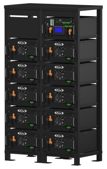
The ET-HV high voltage lithium battery energy storage system consisting of multi battery modules (51.2V200Ah) and a BCU (Battery Control Unit) in series. Single set battery max. supports 17units, with an max. operating voltage range of 185.6V-980V, is used for household / commercial energy storage applications, working with a high voltage inverter for energy storage purposes.
