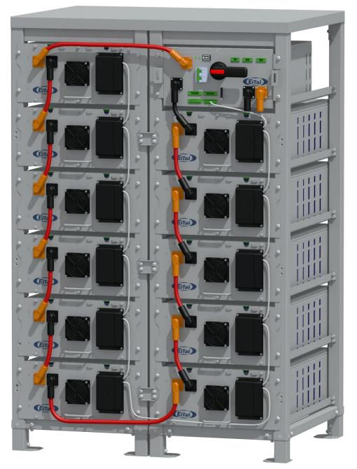
ET-51.2V280Ah-HV high voltage lithium battery energy storage system, consisting of 8-17 battery modules (51.2V280Ah) and a BCU (Battery Control Unit) in series, with an operating voltage range of 358.4V-979.2V, is used for household / commercial energy storage applications, working with a high voltage inverter for energy storage purposes.
