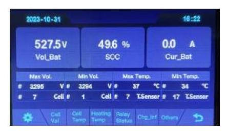
'Cell Vol': single cell voltage;
