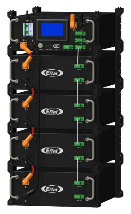
ET-HV high voltage lithium battery energy storage system consisting of multi battery modules (51.2V100Ah) and a BCU (Battery Control Unit) in series. Single set battery max. supports 17units, with an max. operating voltage range of 185.6V-980V, is used for household / commercial energy storage applications, working with a high voltage inverter for energy storage purposes.
