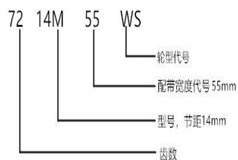
同步带轮基本形状结构图例/Timing belt pulley structure legend
