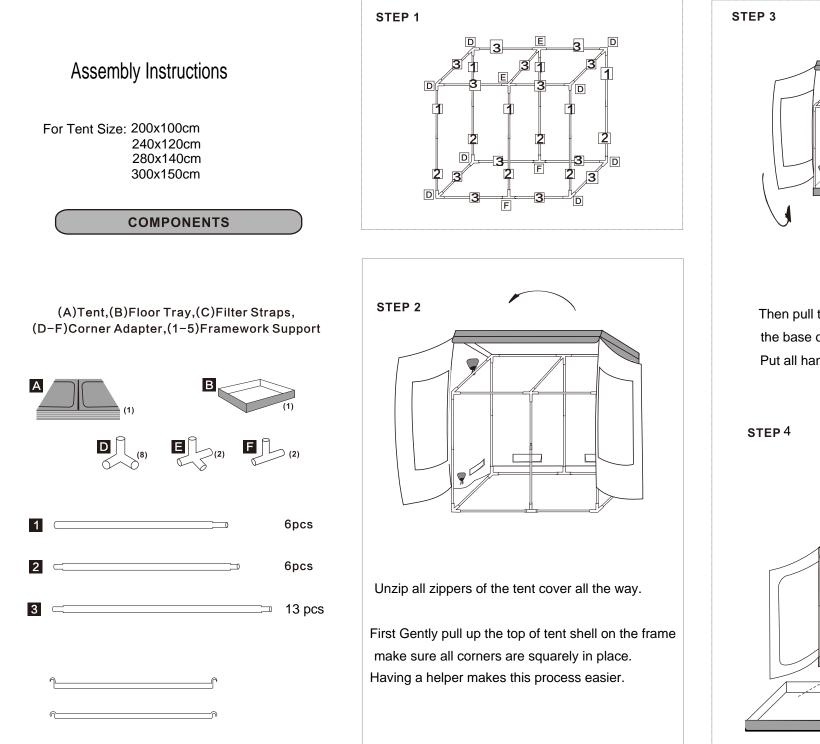
Then pull the bottom of tent shell under the base of tent frame propertly. Put all hanging bars on the top of frame.
