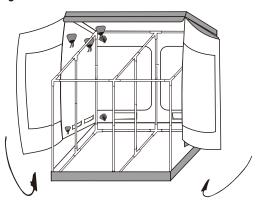
Then pull the bottom of tent shell to cover the base of tent frame propertly.
