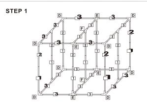
Insert every tube to the bottom of connector.
