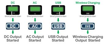
After the screen starts, enter the system. Short press the DC/AC power button to turn on/off the corresponding output. If the AC/DC power button is not turned on, the LCD will automatically shut down after 1 minutes and system will automatically shut down after 8 minutes.
