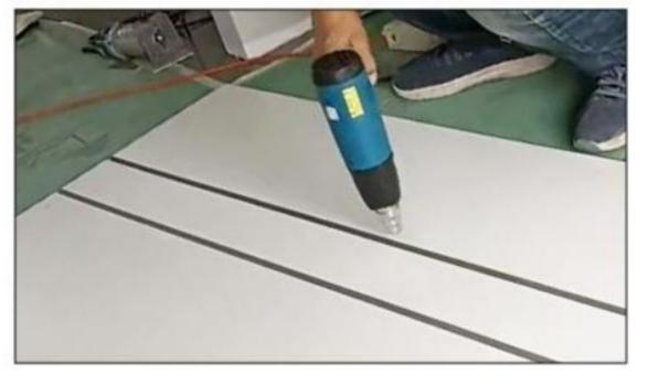
2. Heat the grooved areas evenly with a heat gun, then bend to the desirde angle as the temperature rises.
