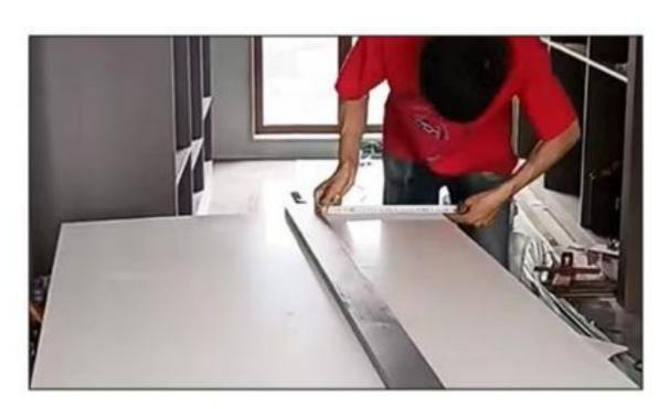
1. Measure with a ruler, mark the position to be bent, and use a grooving machine to make grooves along the marks on the panel.
