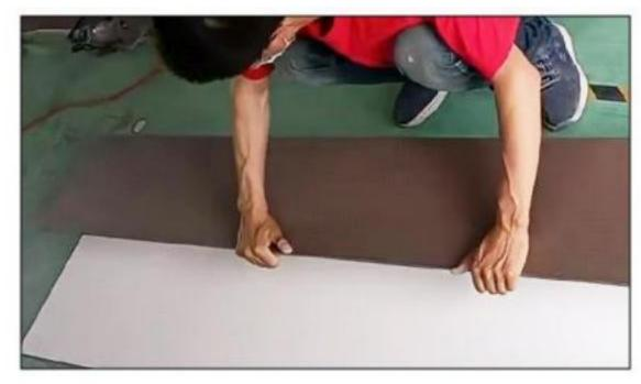
3.Bend to the desired angle, let it sit for a while, and once it cools down and stabilizes, it can be installed.
