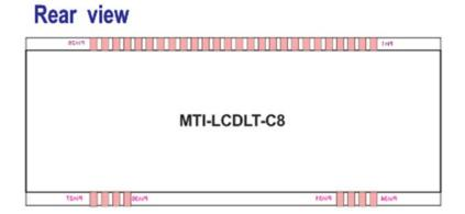
Part No. "MTI-LCDLT-C8" must be printing on LCD back side
