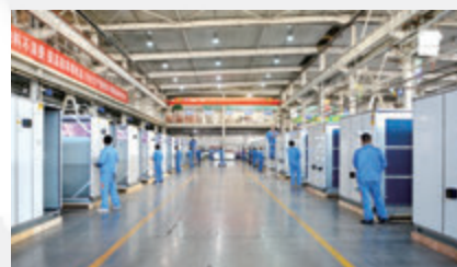
Assembly area of combined air handling unit
