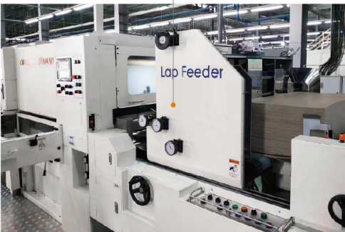
Secondary Positioning Mode: 1. The paperboard is sent from servo vacuum suction belt; 2. Side positioning of single paperboard and front positioning of the back push plate.
