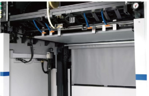
When stripping function is used, this section is high pile stacking section. When finished product feeding function is used, this section is waste collection section.
