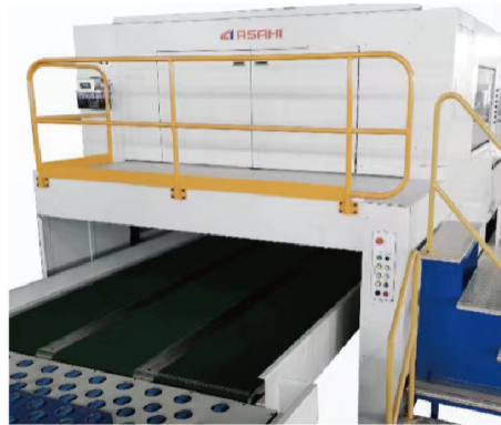
Bundle sheet counting delivery, servo motor control temporary unloading device.
