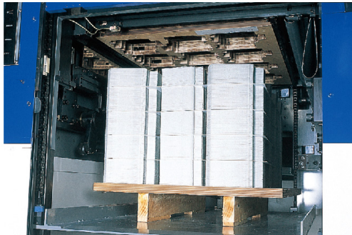
Various boxes such as medicine, cigarette boxes can be stacked neatly by the blanking system. Blanking system and stripping device can be exchanged functionally.
