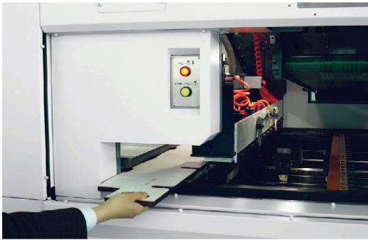
The knock off plate is inserted from outside of the machine on operation side and it can locked by cylinder at one time.
