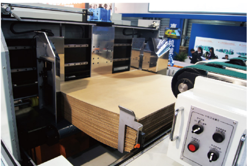
Latest Servo Drive Vacuum Suction Belt Feeding device, eliminates damages to the printed surface.
