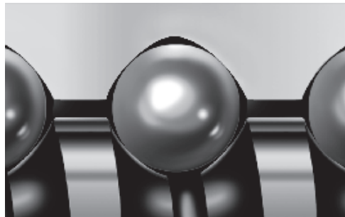
Fig 1.1.2 Groove Shape of YOSO MOTION Precision Ball Screw
