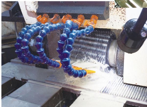
• Milling the rack tooth
