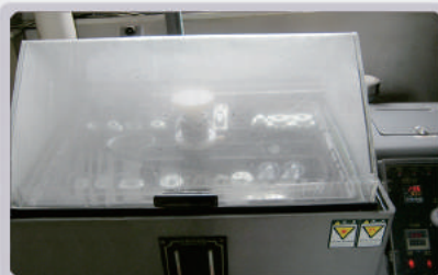
盐雾测试 CORROSION TEST MACHINE
