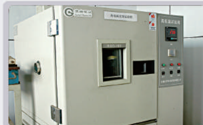
高低温测试 HIGH-LOW TEMPERATURE TEST
