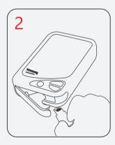
2. Place the filled cuvette in the cuvette holder and push it back
