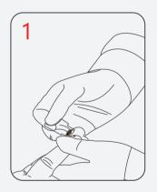
**1**. Fill the cuvette by placing the tip of the cuvette in the drop of blood.
