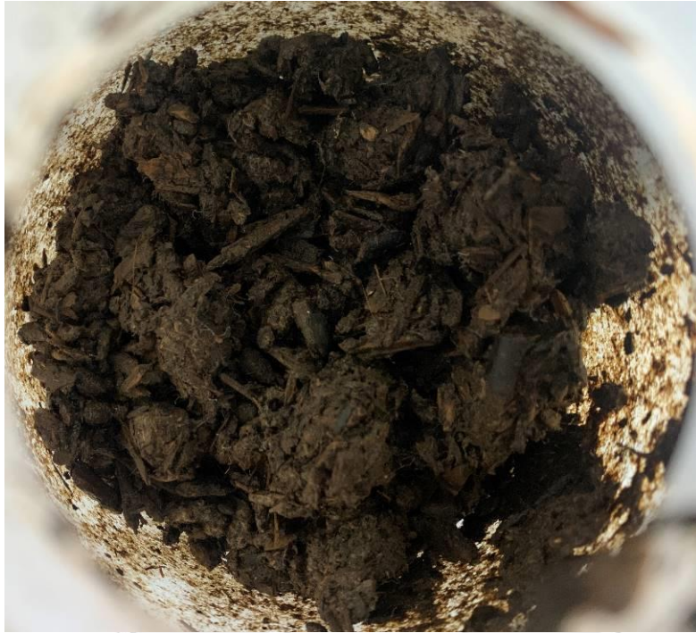
Fig 5.The mixture of test item and inoculum at the end of the test (45days,vessel 1)
