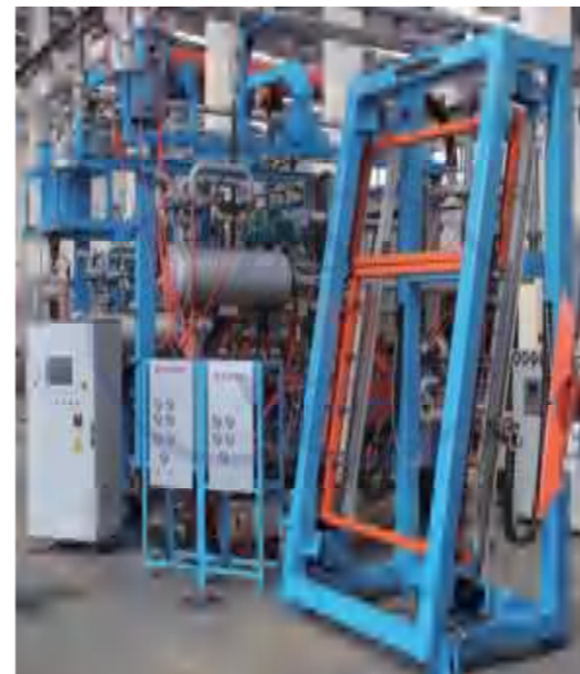
振动切割和自动调丝机构 vibrating cutting and wire auto adjusting system
