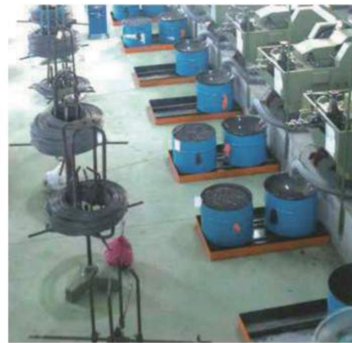
Heading machine to form screws
