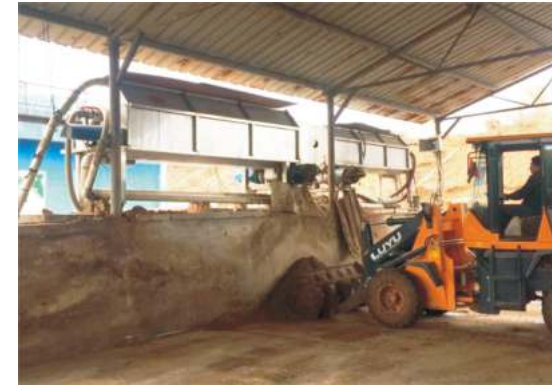
Use different size of screen to process multi-stage filtration
