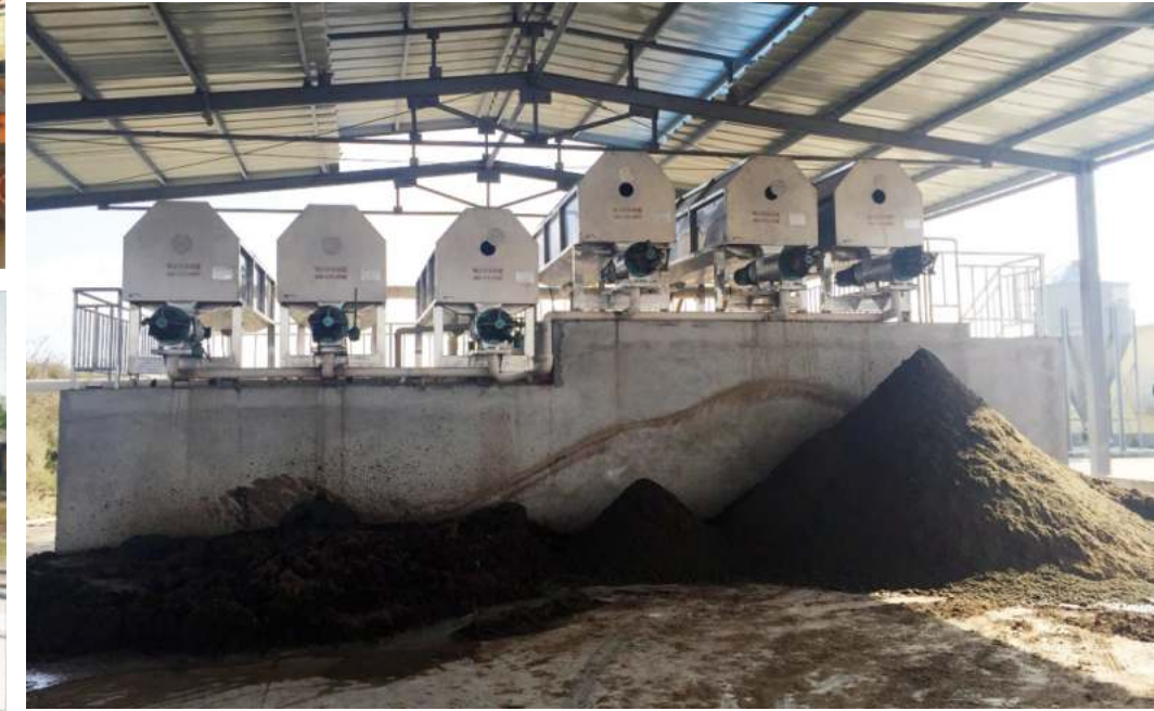
Use different size of screen to process multi-stage filtration
