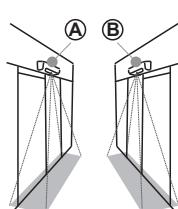
When installing two sensors in adjacent areas, please separately choose channel A and channel B to avoid mutual interference and misoperation.
