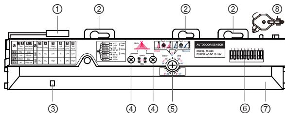
① Connector   ② Installation hole   ③ Action indicator light   ④ Safety width adjustment screw
