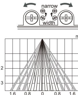
Microwave sensitivity adjustment: high, middle, low, ultra-low, a total of 4 levels. High sensitivity with the maximum detection range, ultra-low sensitivity with the minimum detection range.
