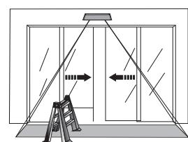
After continuously hold for 15 seconds(15s,1min,30min are optional), no other objects or human bodies appear in the detection range, the system will automatically learn the static object as the new background. And it will no longer trigger the door opening signal, and automatic door will close back automatically(As the picture shows).
