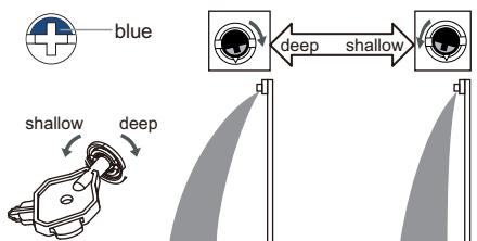
The left & right width screws is used to adjust the induction width, with narrow and wide two levels.
