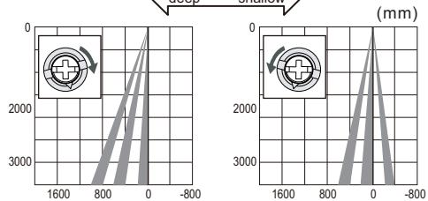
The blue screw is used to adjust the depth of microwave induction. Turn clockwise will away from the door. Turn counterclockwise will close to the door.
