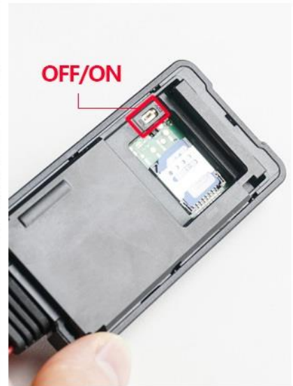
Step 3: Push to the right to close the slot Turn ON the switch
