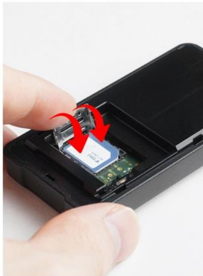
Step 2: Pan to open the card slot and Insert your SIM card
