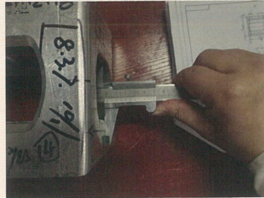
壁厚检查/ Wall thickness check
