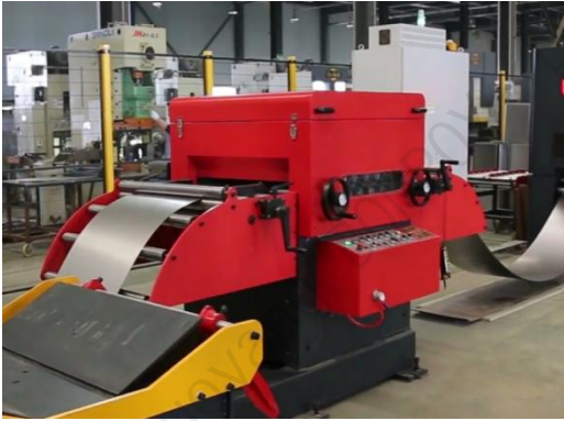
➤ Steel plate leveling
