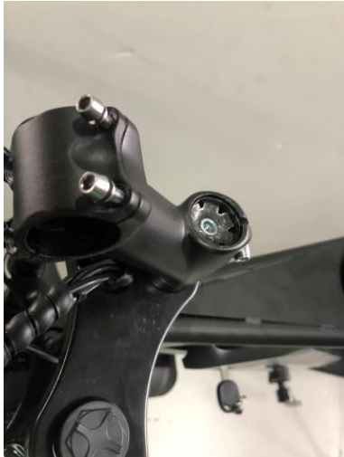
7. Take out the handle holder from the tooling kit and put it into the round tube of front fork
