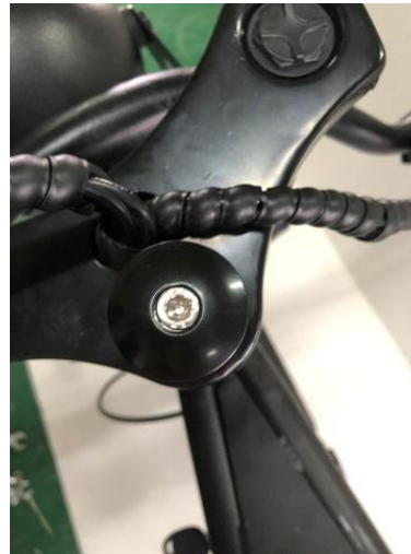
5. Use the M5 Allen wrench to unscrew the screw
