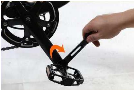
25. Use the 13-15 wrench to tighten the pedal(same on both sides)
