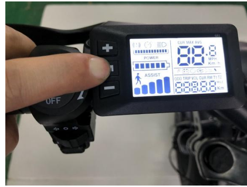
27. Press and hold the M button for 3 seconds to turn it on
