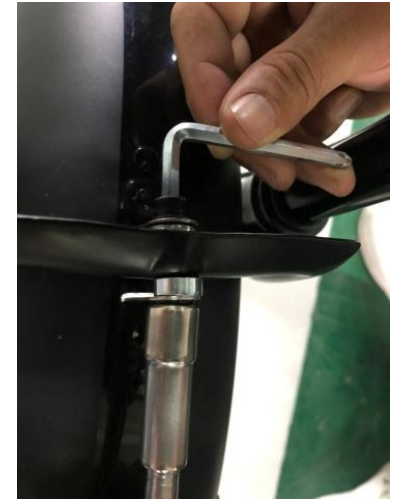
18. Tighten the screws until the front fender is not movable.
