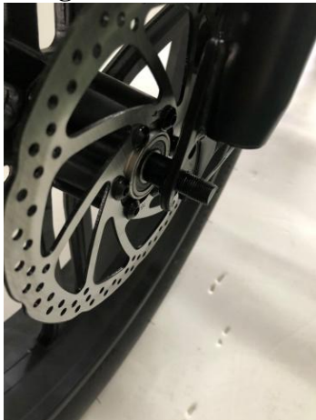
19. Take out the disc brake from the tool box and install it on the front wheel, then insert the front wheel into the front fork slot
