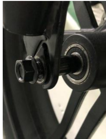
20. Place small parts according to the sequence in picture (same on both sides)
