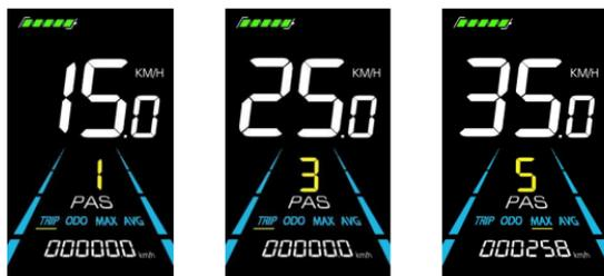
Figure 5-4 PAS level display interface
