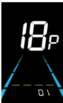
Figure 6-18 6km/h walk boost setting interface
