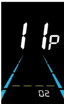
Figure 6-11 Pedal assist sensitivity setting interface
