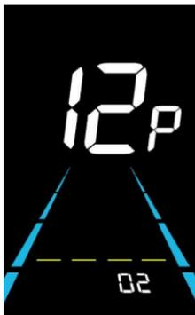
Figure 6-12 Pedal assist Start-up intensity setting interface
