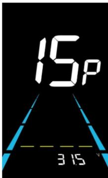
Figure 6-15 Battery under voltage value setting interface
