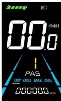
Figure 5-3 Backlight display interface
