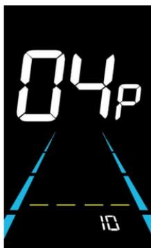
Figure 6-4 Auto Power Off Time Setting Interface
