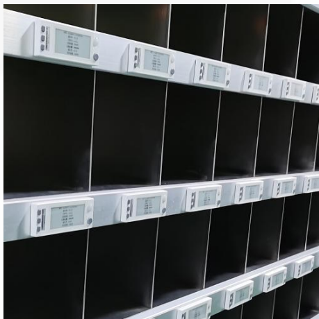
Warehouse light picking
