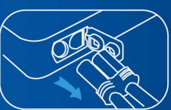
Remove the plug from the jump starter then remove the clamps
