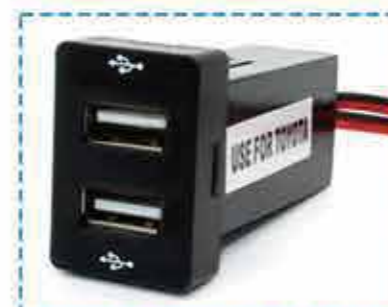
YJ-STUB006B-1 Dual Small Toyota USB Input: DC12-24V Output: 5V/4.2A Material: ABS+Copper Hole size: 32*20*70mm
