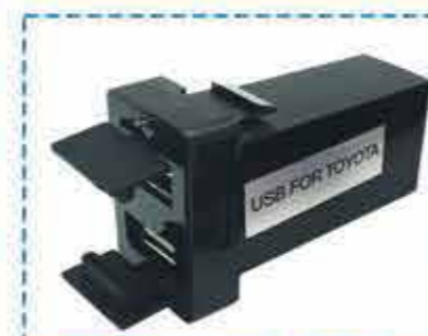
YJ-STUB006B Dual Small Toyota USB Input: DC12-24V Output: 5V/4.2A Material: ABS+Copper Hole size: 32*20mm
