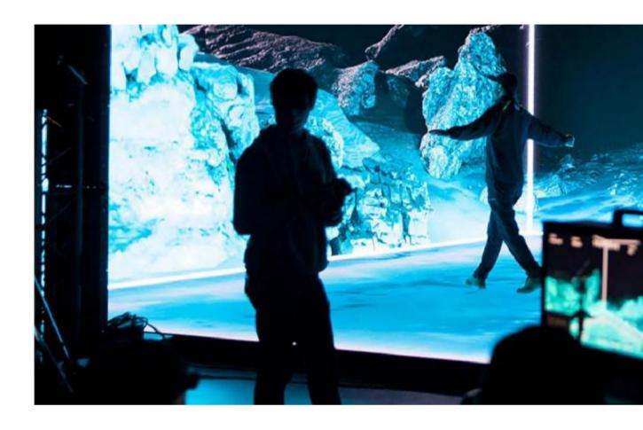
The MGF series is a digital solution with high load-bearing capacity, quick disassembly, and increased cabinet protection. The anti-re active and anti-slip surface provides perfectly uniform blacks and great visual performance under any light condition and at wide viewing angles. The MGF series allows it to carry up to 1500kg/m2.
