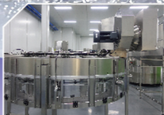
空瓶无菌风送系统 Empty Bottle Sterile Air Delivery System 产能 Capacity: 95 m/min
