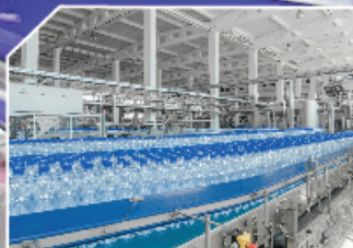
瓶输送系统 Bottle Transfer System 产能 Capacity: 6000-72000BPH
