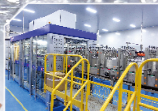
热收缩膜包装系统 Shrink-wrapper System 产能 Capacity: 120packs/min
