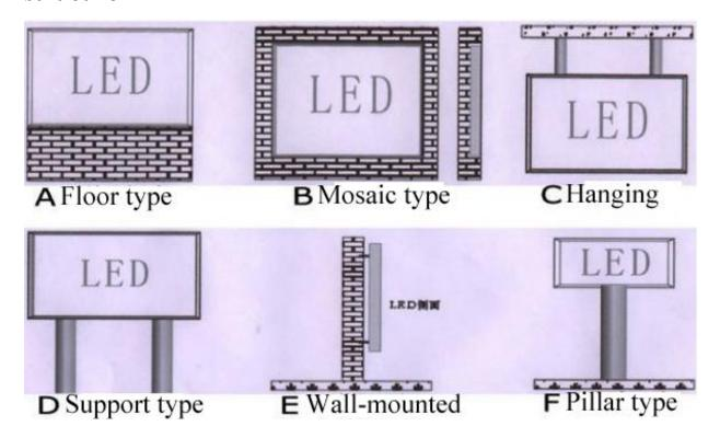
Note: The above are the six installation methods commonly used in the installation of the display screen at present. For the indoor display screen, the four installation methods A\B\C\D are generally adopted, and the above methods can be used for the outdoor display screen.
