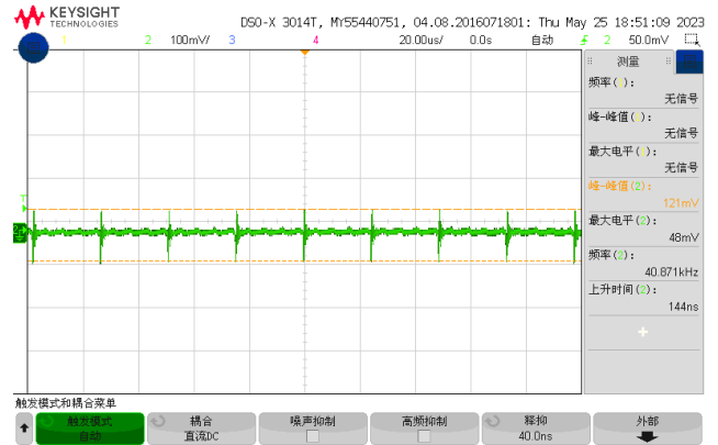
Figure 7, Output ripple & noise (Iout = 15A)
