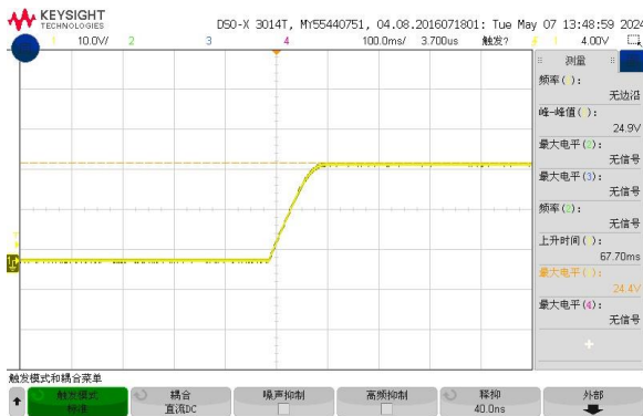
Figure 6, Output voltage established (Iout = 40A)
