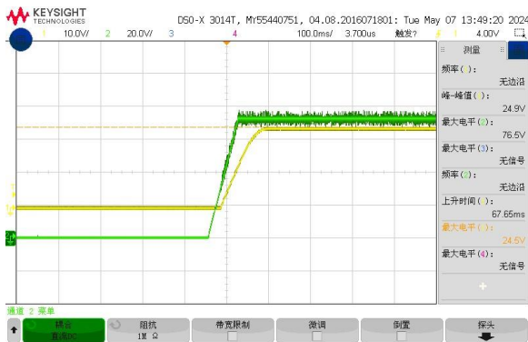
Figure 8, Boot delay time (Iout = 40A)
