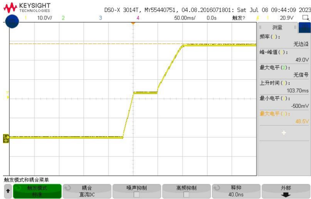
Figure 6, Output voltage established (Iout = 32A)
