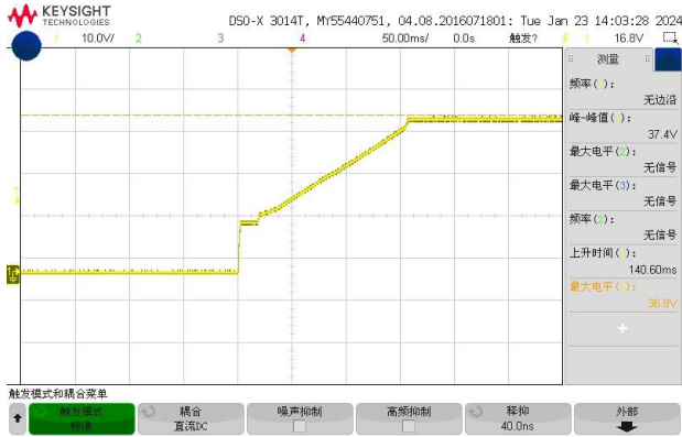
Figure 6, Output voltage established (I out = 15A)
