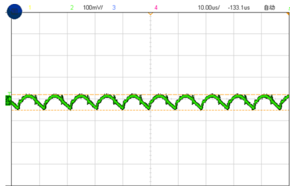
Figure 7, Output ripple & noise (Iout = 3A)
